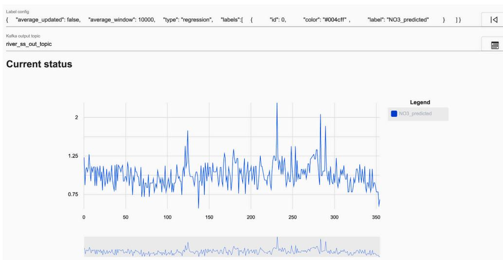
Fig. 6. Real-time  $\text{NO}_3^-$  contents soft sensor prediction visualisation in Kafka-ML.
