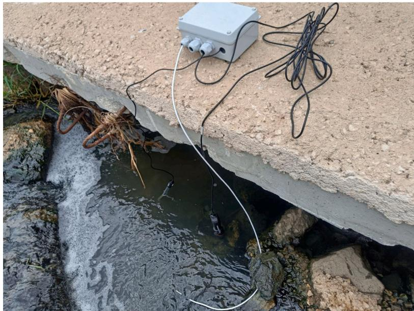
Fig. 5. IoT prototype deployment for soft sensor in the Guadalhorce river (Málaga, S Spain).
